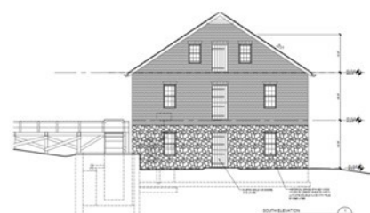
South elevation showing wheel pit and entrance off Mill Stone Trail.
