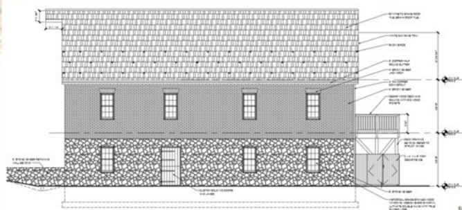
East elevation with view of entrance adjacent to walking trail. Mill building is to be three stories with additional door on the south elevation at grade and a third entrance via ramp to the second floor at the north.
